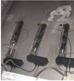
Complete actuator system exposed to ice water (ISO 16750-4) and Arizona dust (ISO 20653).
