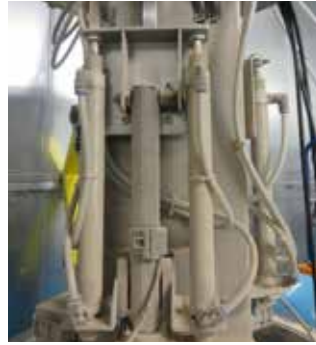
Extensive duration tests have validated a life target of more than 17 000 cycles over 15 years
